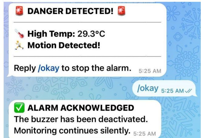
Figure 10. Telegram alert triggered by elevated temperature combined with motion detection, followed by user acknowledgement.
