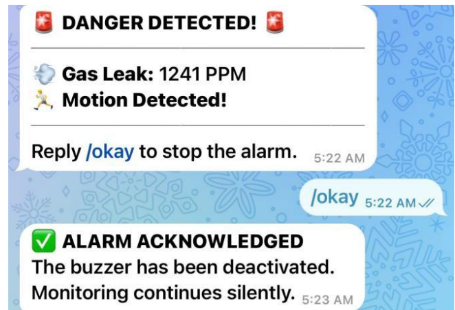
Figure 9. Telegram alert generated when the programmed MQ-2 threshold and PIR motion input were simultaneously present.
