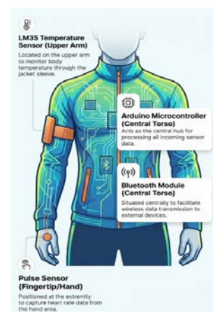
Figure 5. Component placement and wearable implementation of the IoT Fitness Jacket
