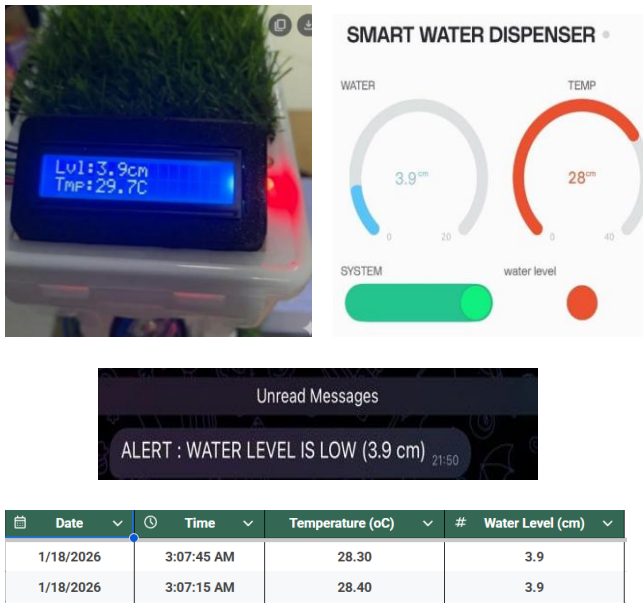
Figure 6. Integrated low-water condition response showing local LCD warning, Blynk dashboard visualization, Telegram alert notification, and Google Sheets data logging.
