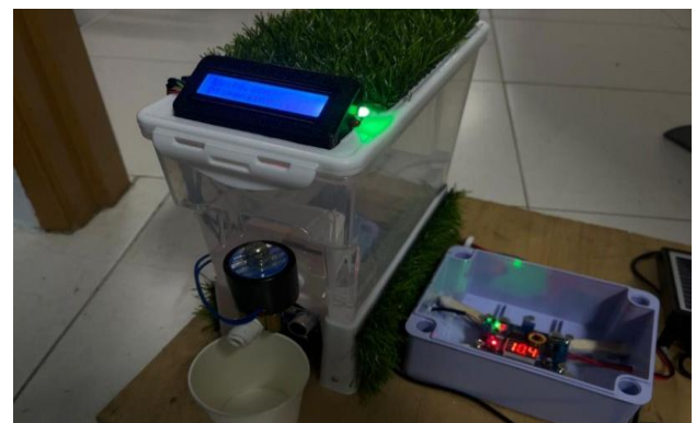
Figure 3 The completed prototype of Smart Contactless Water Dispensing and Monitoring System with Dual-Platform Notification via Blynk and Telegram.
