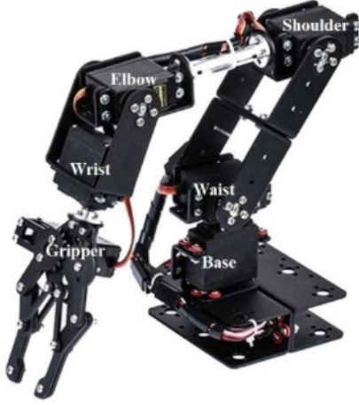
Figure 2. Six degrees-of-freedom (6-DoF) robotic arm prototype constructed with ABS frame and MG996R servomotors
