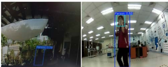
Figure 8. Detection performance under varied lighting conditions: (Left) Low-brightness environment; (Right) Bright environment
