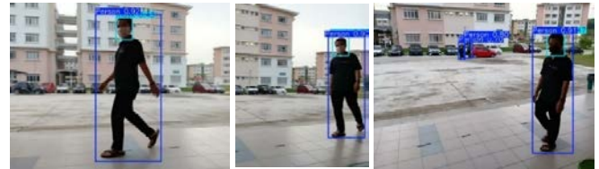
Figure 9. Detection performance in an open space under adequate lighting conditions: (Left) A moving person at less than 5 meters; (Middle) A person wearing a bright mask at 5 meters; (Right) A person wearing a dark mask at 5 meters
