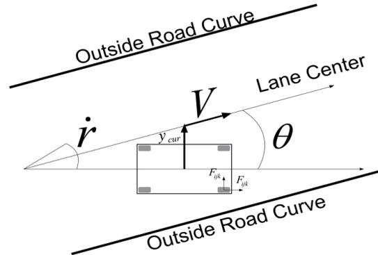
Figure 2: The illustration of kinematics model for the vehicle.
