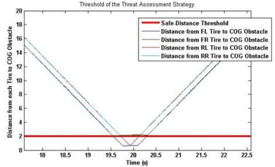
Figure 3: Once the safe-distance threshold has been violated, GMC-VCA block will be activated.
