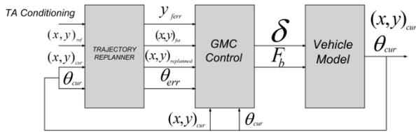
Figure 4: Overall architecture of VCA system. The GMC will be activated once the TA-threshold is violated.
