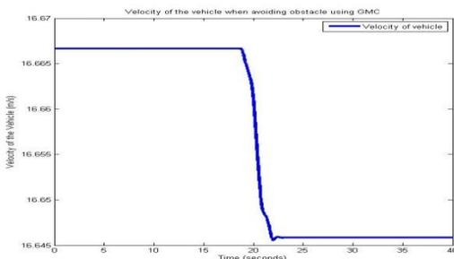
Figure 8: Vehicle Velocity while avoiding obstacle using GMC Method.
