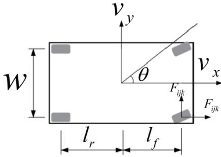
Figure 1: The illustration of 3-DOF vehicle model used in this work.
