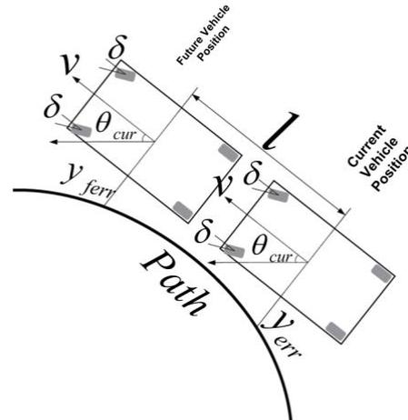
Figure 5: Coordinate of host and current vehicle to find the future lateral error.
