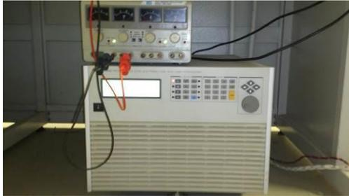
Figure 1: Experimental setup for Ni-MH battery
