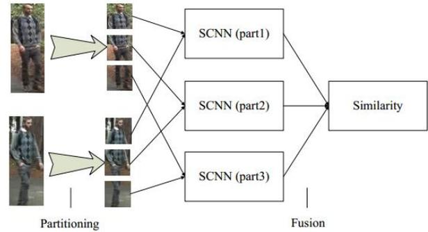
Figure 7: Flowchart of Siamese Convolution Neural Network [38].
