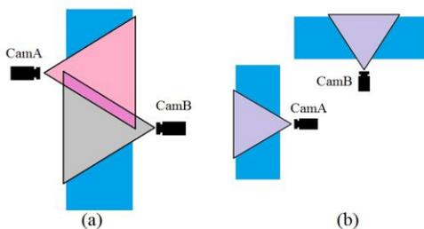
Figure 2: Typical camera setup for: (a) overlapping views and (b) non-overlapping views.
