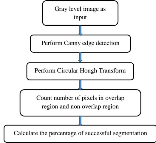
Figure 3: Flow diagram of segmentation implementation
