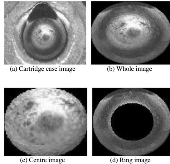
Figure 4: Segmentation of firing pin impression into three parts manually (b), (c) and (d)
