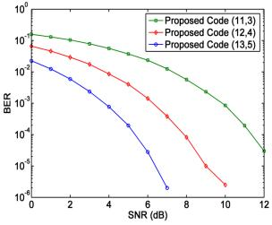
Figure 5: BER performance versus SNR for several proposed codes
