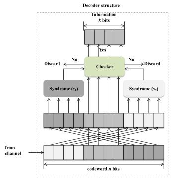
Figure 2: Decoder structure for the proposed code
