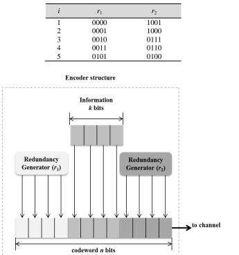
Figure 1: Encoder structure for the proposed code
