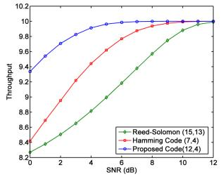
Figure 6: Throughput performance versus SNR for the proposed code, Reed Solomon and the Hamming code
