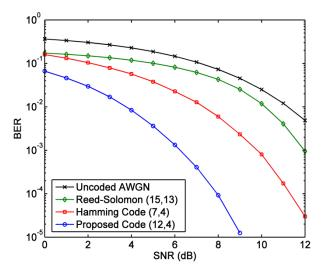
Figure 4: BER performance versus SNR for the proposed code, Hamming code and Reed-Solomon code
