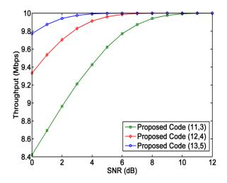
Figure 7: Throughput performance versus SNR for the proposed codes with various codeword lengths
