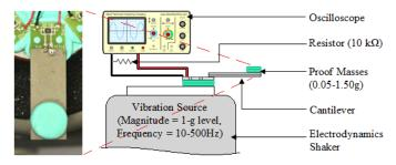
Figure 4: Illustration of the Experiment Set-up for Proof Mass Variation
