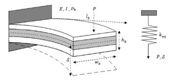
Figure 1: Illustration of Measurement Variables of Piezoelectric Cantilever
