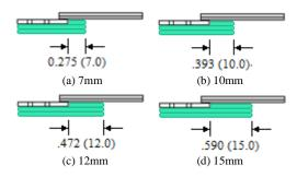
Figure 5: Illustration for Reducing Cantilever Length by Clamping Over
