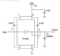
Figure 7: MOSFET Driver Circuit using TC4422
