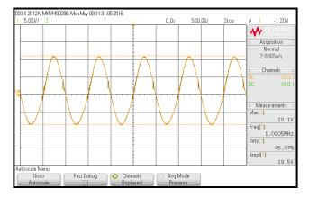
Figure 14: Output Voltage from Class E Inverter
