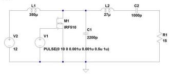
Figure 8: Class E Inverter
