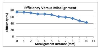
Figure 18: Graph of Efficiency vs Misalignment
