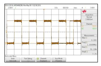
Figure 12: Output Waveform for MOSFET Driver
