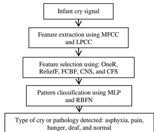
Figure 1: Block diagram of the automatic infant cry classification system
