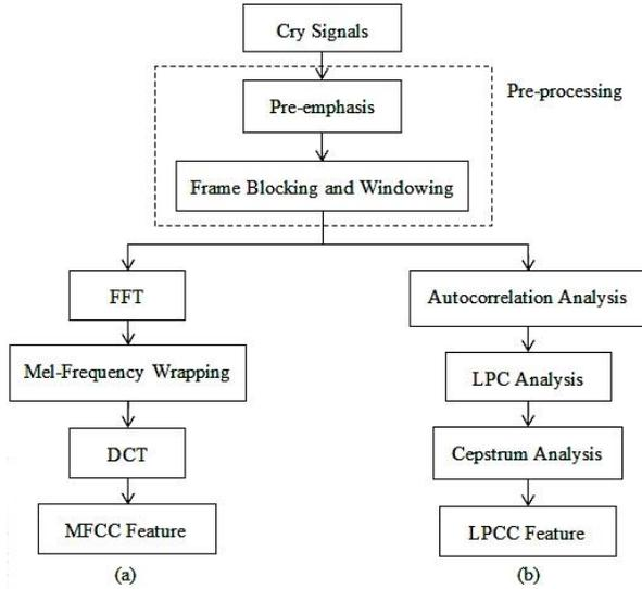
Figure 2: Block diagram of features extraction process: MFCC feature (a) and LPCC feature (b)
