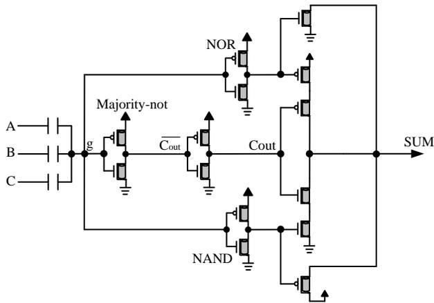
Figure 6: The schematic of SyMuT cell [9]
