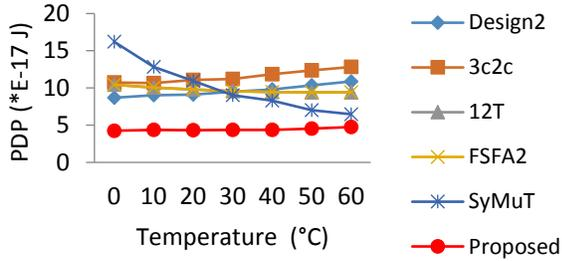
Figure 9: PDP versus temperature (supply voltage=0.5V, frequency=100MHz, C<sub>load</sub>= FO4)
