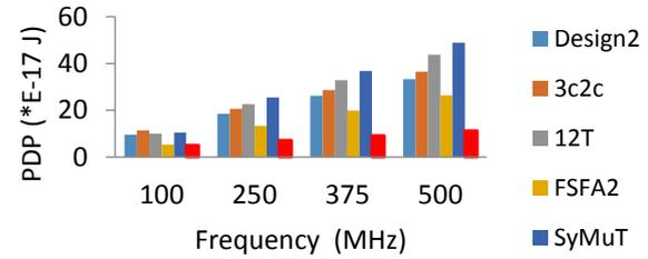
Figure 11: PDP versus input operating frequency (supply voltage= 0.5V, C<sub>load</sub>= 0.5fF)
