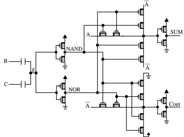
Figure 5: The schematic of FSFA2 cell [8]
