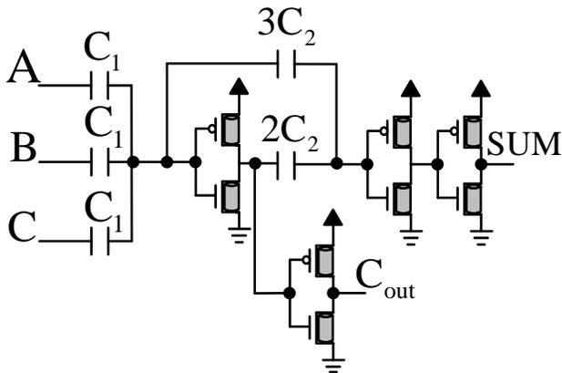
Figure 3: The schematic of 3c2c cell [6]
