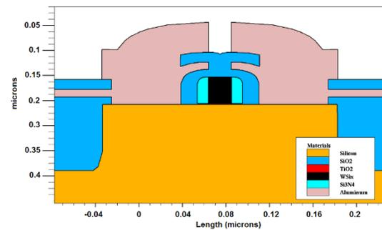
Figure 2: Completed PMOS transistor with 22 nm gate length
