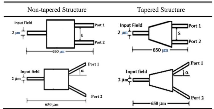
The effect of electric field intensity of each structure is observed. The results show that when the separation distance is in the intermediate value, the electric field intensity is at the highest. Furthermore, the electric field intensity increases, while the arm angle is increasing. Besides, the tapered MMI structure gives a better electric field intensity rather than the typical MMI design structure.
