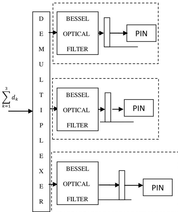
Figure 3: ZCC code receiver system
