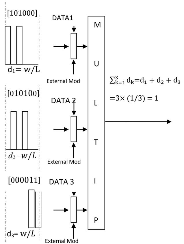
Figure 2: Block diagram of a new ZCC code transmitter system.
