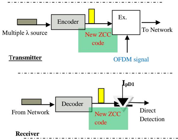
Figure 1: Scheme illustrates the (OFDM-OCDMA) system
