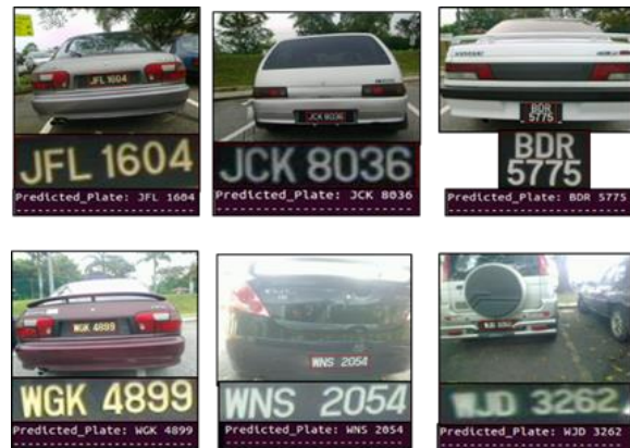
Figure 5. Successful plate detection and character recognition in challenging conditions
