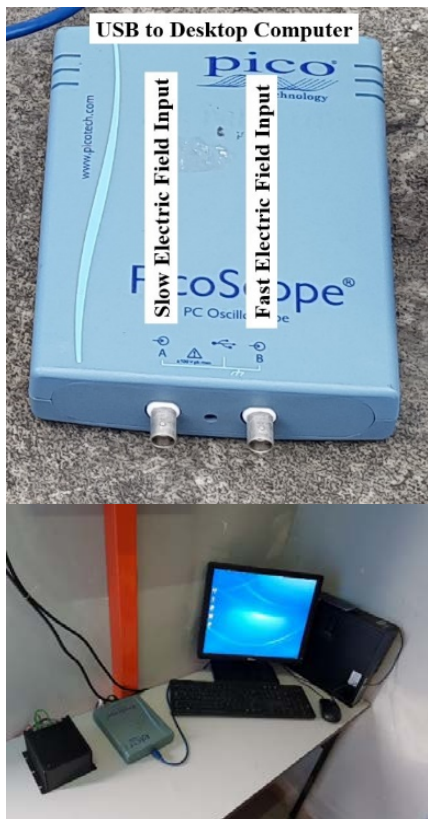
Figure 5. PicoScope 4000 series, AC-DC power supply -12VDC +12VDC and desktop computer with PicoScope 6 software installed
