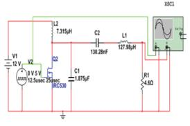
Figure 3: Class-E converter design circuit
