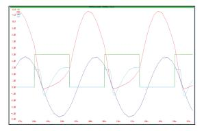
Figure 8: ZVS condition for Class-E circuit
