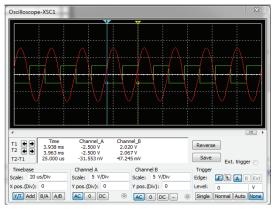
Figure 6: Oscilloscope output at f = 40 kHz (Ch. A - VGS, Ch. B - Output)
