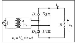
Figure 4: Schematic diagrams of Rectifier circuit design [13]
