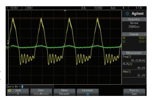
Figure 12: Oscilloscope Result Taken After Metal Block At The Transducer Receiver
