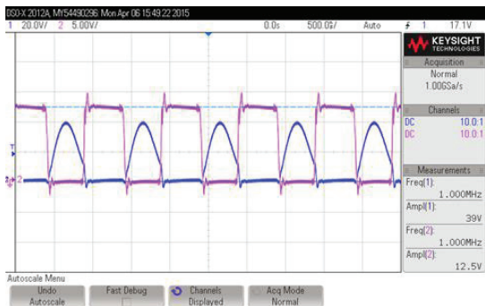
Figure 9: Drain V_D (Blue) vs. Gate V_G (Purple) ZVS [Practical]
