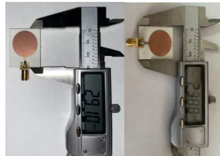
Figure 9. The dimension of Fabricated Antenna (a)Length (b)Width
