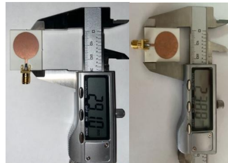
Figure 9. The dimension of Fabricated Antenna (a)Length (b)Width
