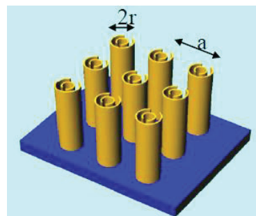
Figure 1: Array structure of split ring resonator by [3] with 2r and a dimension
