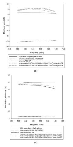
Figure 5: Simulated results of the antenna in various scenarios (a) Return loss (b) Realized gain (c) Radiation efficiency
