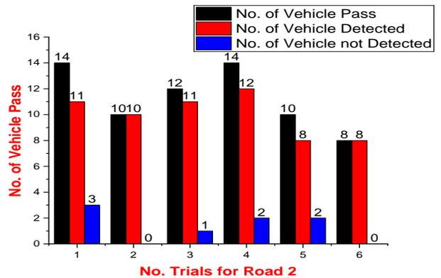
Figure 10: Performance measurement for Road 2 with IR Sensor
