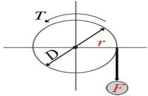
Figure 4: Torque of servomotor
