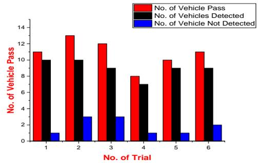
Figure 9: Performance measurement for Road1 with IR Sensor
