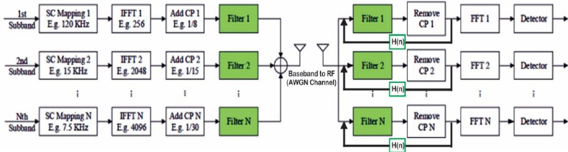
Figure 3: Block Diagram of FF-OFDM Transceiver System
