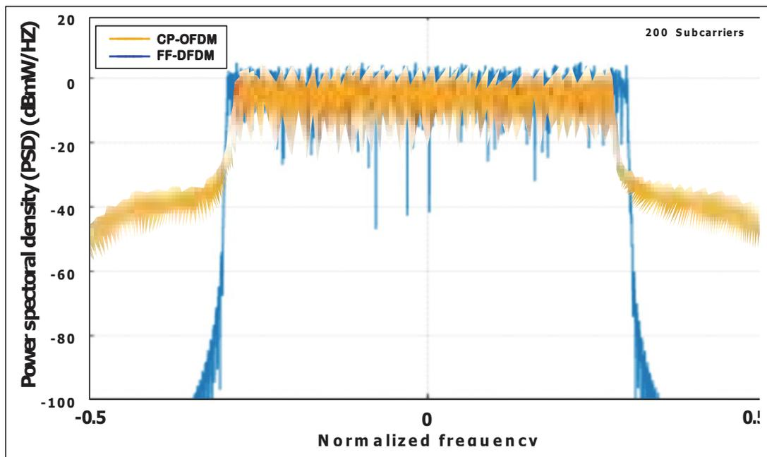
Figure 7: Comparison of Generated FF-OFDM and CP-OFDM Waveforms
