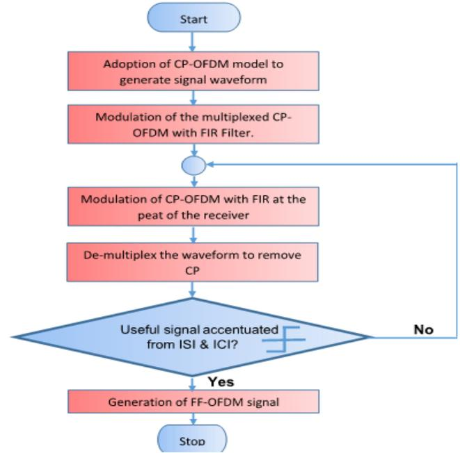
Figure 5: FF-OFDM Signal Waveform Generation Flowchart
