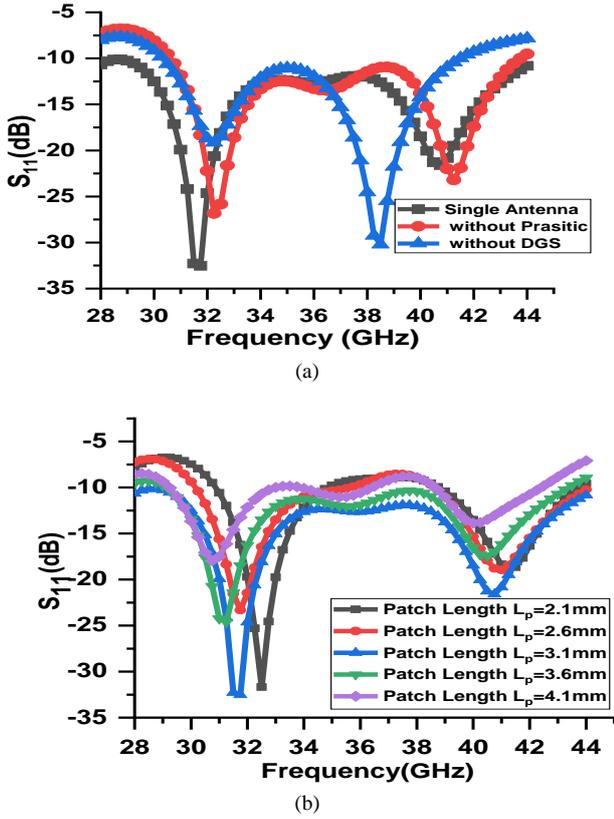
Figure 2: (a) S11 plot of the proposed single antenna element, without DGS and without parasitic element (b) Antenna parametric analyses on variation of the length of the radiating patch
