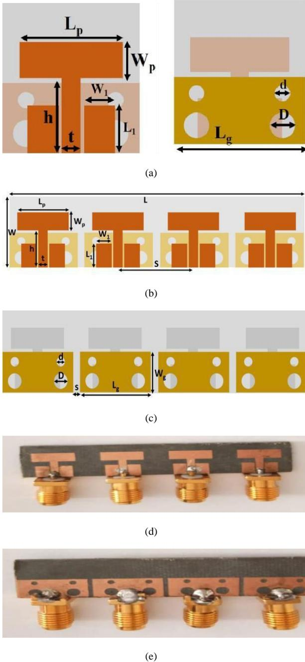
Figure 1: (a) Layout of single antenna element, Proposed MIMO antenna layout (b) Front view (c) Back view, Fabricated MIMO antenna (d) Front view. (e) Back view
