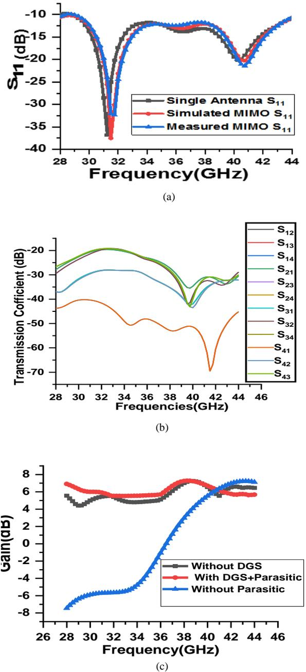
Figure 3: (a) Comparison of simulated and measured return loss (b) Measured Transmission coefficient of the proposed MIMO antenna (c) Gain of single antenna element, without DGS and without parasitic element
