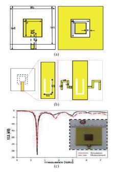
Figure 4: Proximity coupled antenna harmonic suppression; (a) Geometry antenna structure both front and back view; (b) Symmetrical inverted arm stub with U-slot on feedline; (c) Validated result of simulation and measurement [42]
