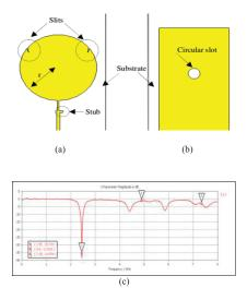
Figure 6: Circular patch antenna, (a) Top view; (b) Bottom view; (c) Return loss [45]
