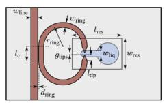
Figure 1: Geometrical parameters of the coupled DR-SRR sensor [2]
