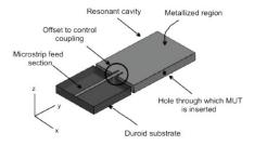
Figure 2: Layout of substrate integrated waveguide cavity resonator with microstrip feed section and hole within the cavity through which the MUT is inserted [7]
