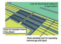
Figure 4: Schematic view of gas-liquid separated resonator [23]
