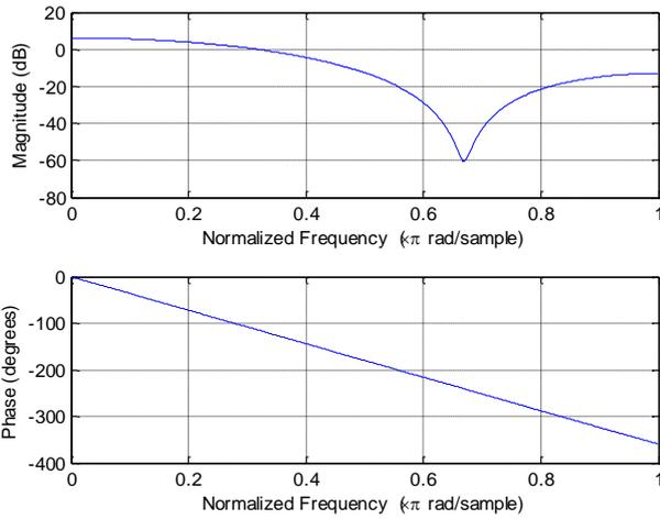
Figure 4: Frequency response of the Proakis C channel
