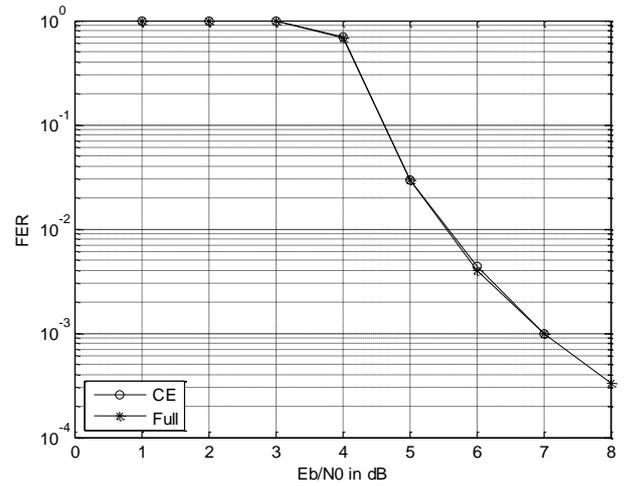
Figure 6: Frame Error Rate (FER) of MAP-CE and MAP-Full turbo equalizers
