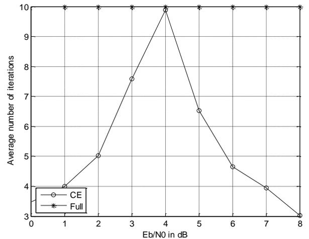
Figure 7: Average number of iterations of the MAP Turbo equalizer using the CE criterion
