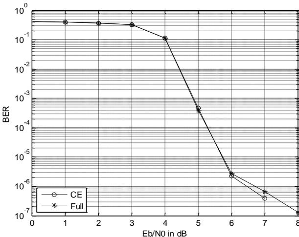
Figure 5: Bit Error Rate (BER) of MAP-CE and MAP-Full turbo equalizers.
