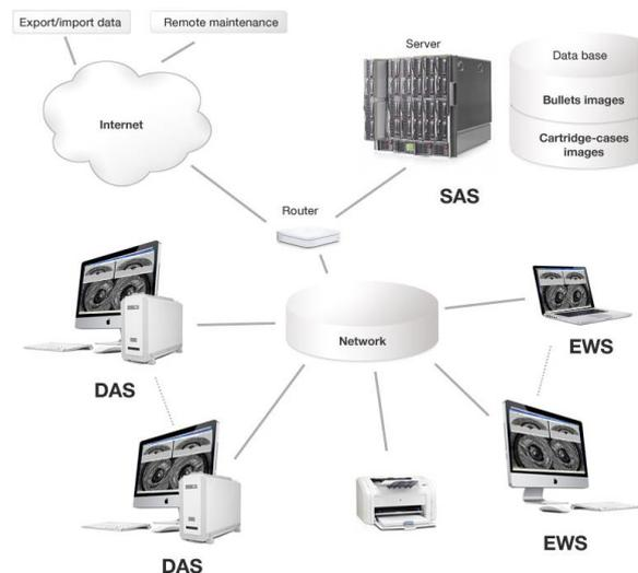
Figure 1: The components of the Evofinder system
