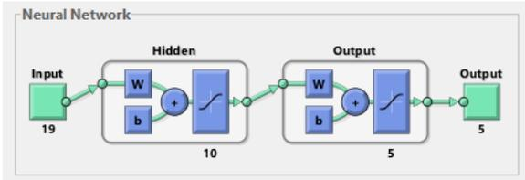
Figure 4: A two-layer feed-forward neural network architecture
