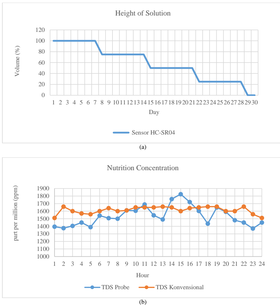
Figure 5: Data on test results for (a) height of solution, and (b) concentration in nutrition
