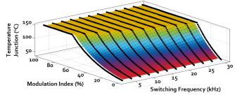
Figure 8: Temperature junction versus switching frequency and modulation
