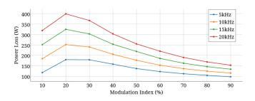
Figure 3: Switch power losses versus switching frequency and modulation index (200V input voltage)
