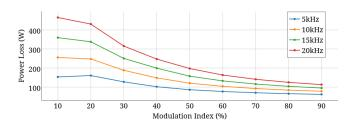
Figure 4: Switch power losses in 300V input voltage
