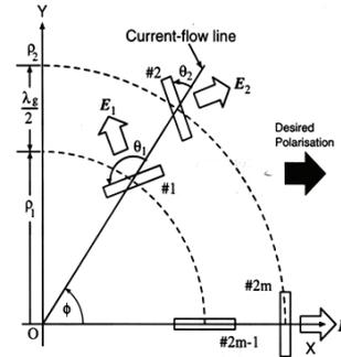
Figure 2: Design of unit radiator of linear polarization.
