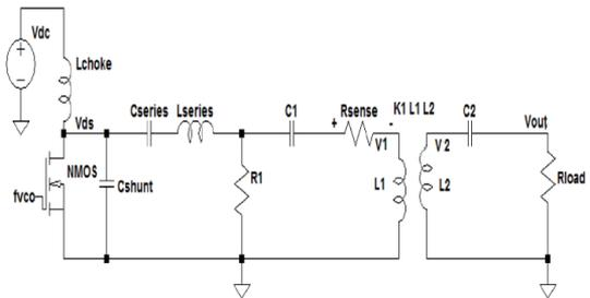
Figure 3: Class E resonant power converter circuit with inductive links
