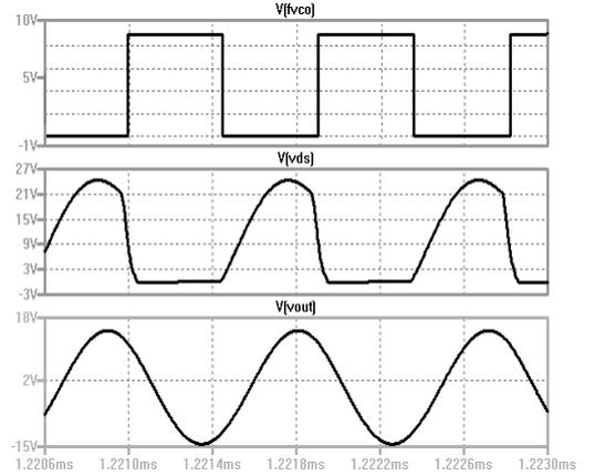
Figure 6: Output waveform of IPT system without frequency tracking
