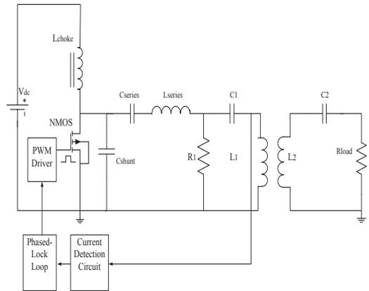
Figure 1: General block diagram of IPT system
