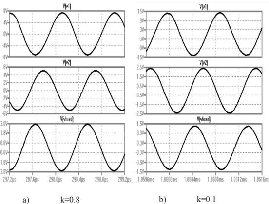
Figure 8: Inductive links without frequency tracking
