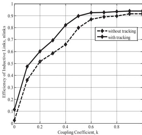
Figure 10: Efficiency of inductive links versus coupling coefficient
