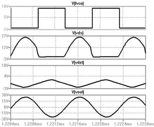
Figure 7: Output waveform of IPT system with frequency tracking
