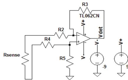
Figure 4: Current sensing circuit
