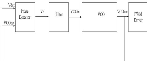
Figure 2: Phased lock loop illustration
