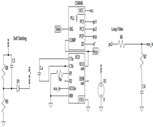
Figure 5: Phased lock loop and its external circuit
