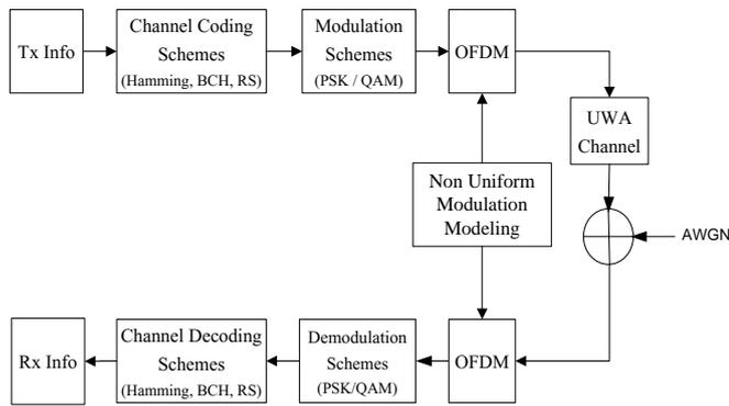
Figure 1: Block diagram of adaptive code with Non-uniform Modulation
