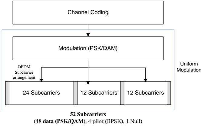
Figure 2: Modeling of the existing standards on OFDM Subcarriers
