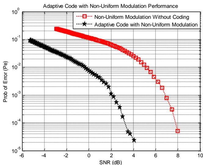
Figure 6: Performance of Adaptive Code with Non-uniform modulation and Non-Uniform Modulation without coding
