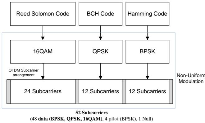
Figure 3: Modeling of the Adaptive Code with Non-Uniform Modulation on OFDM Subcarriers
