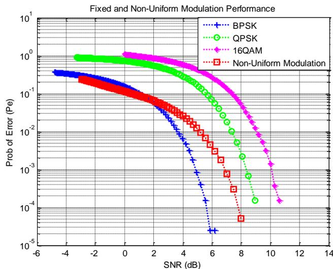
Figure 5: Performance of fixed and Non-uniform modulation
