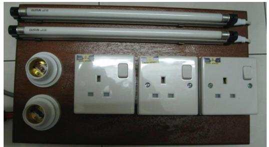
Figure 21: Appliance Board Top View. The board features two 8W fluorescent, two 20W light bulbs and three three-pin switches
