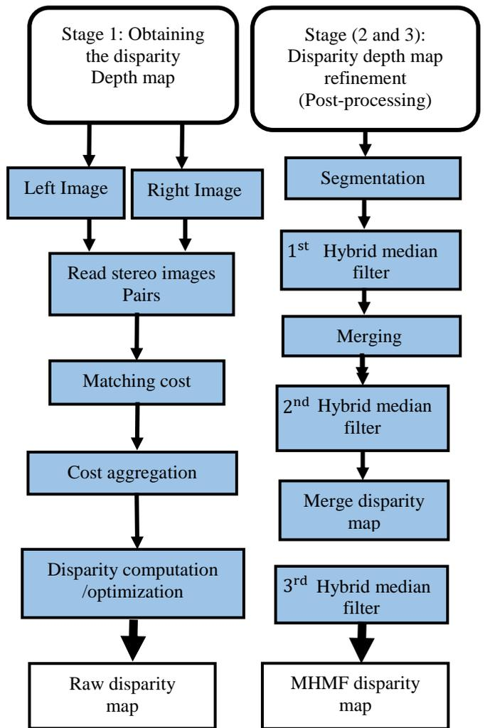
Figure 1: Block diagram and structure of MHMF algorithm
