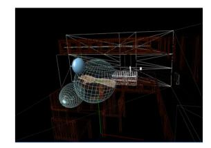
Figure 13: Collision detection with bounding spheres
