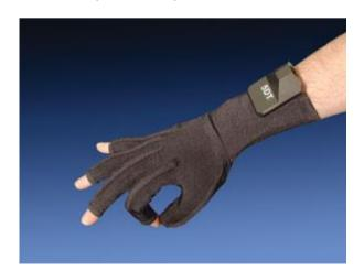
Figure 1: 5DT data glove for hand motion tracking
