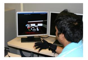
Figure 21: Real-time hand deformation using 5DT data glove
