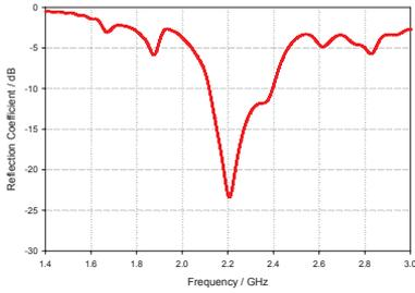
Figure 4: Reflection Coefficient for the Patch Antenna
