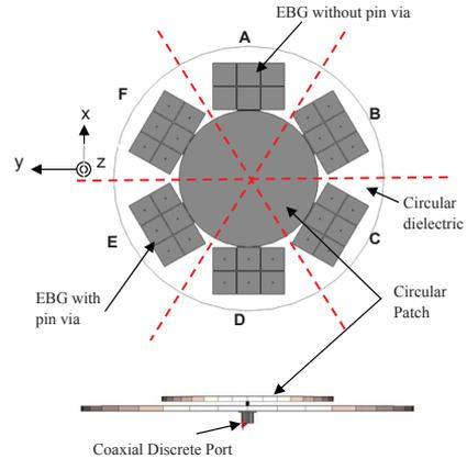
Figure 3: Patch antenna at the centre of an EBG
