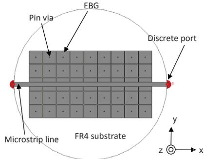
Figure 1: Microstrip transmission line to measure EBG surface mutual coupling
