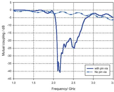
Figure 2: Mutual coupling for a square EBG using microstrip transmission line.
