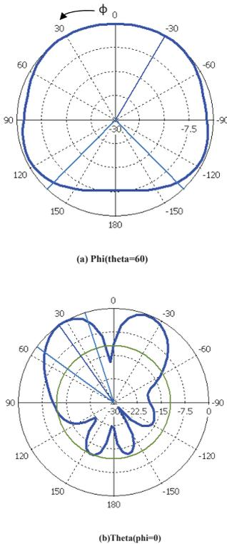
Figure 5: Antenna Power Pattern at 2.2GHz for sector A without pin vias.
