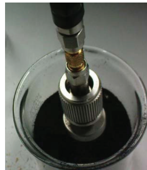
Figure 5: Dielectric properties of measurement of the pure tire rubber dust using dielectric probe technique
