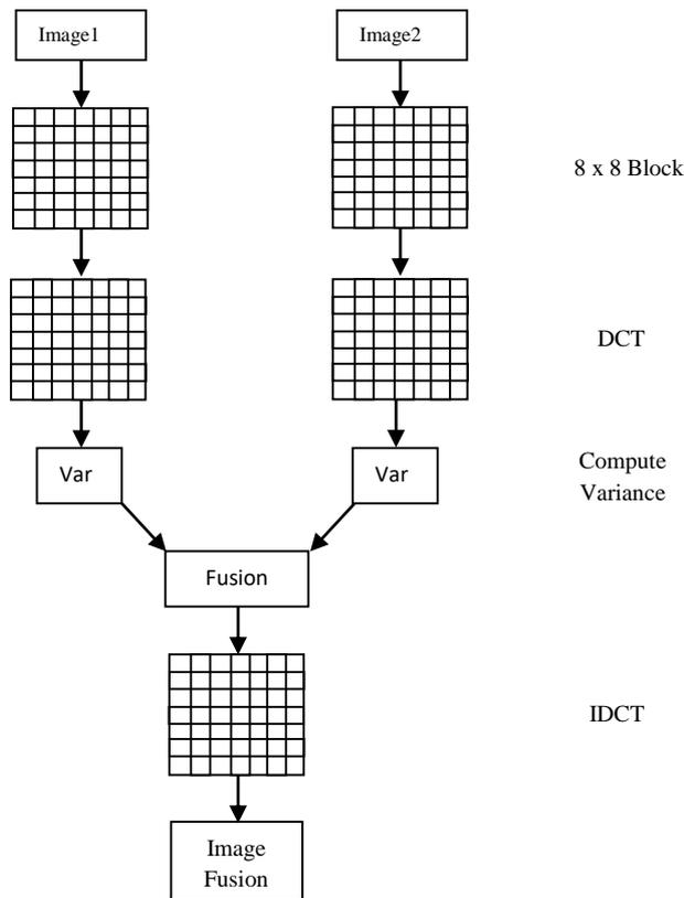
Figure 4: Image Fusion using DCT technique
