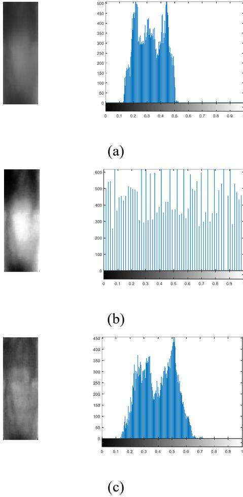
Figure 2: (a) original image and its Histogram, (b) the preprocessed image with Histogram equalization and its Histogram (c) the preprocessed image with CLAHE and its Histogram
