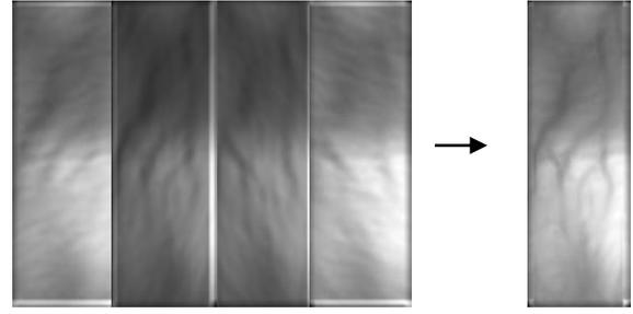
Figure 3: Filtered images with four orientations:  $22.5^\circ$ ,  $67.5^\circ$ ,  $112.5^\circ$  and  $157.5^\circ$ , and the reconstructed image
