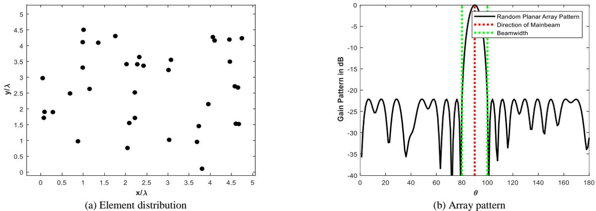
Figure 2: Random planar array pattern and its element distribution
