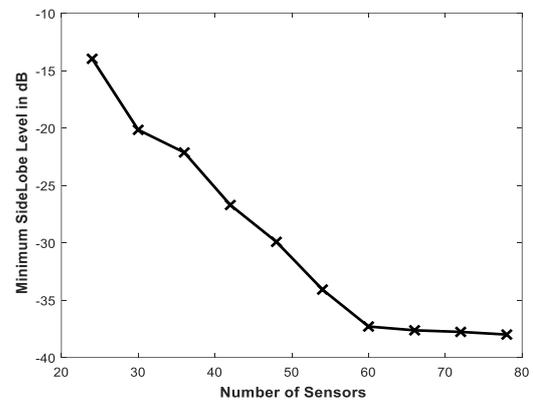
Figure 6: Variations of minimum sidelobe level versus number of sensor elements
