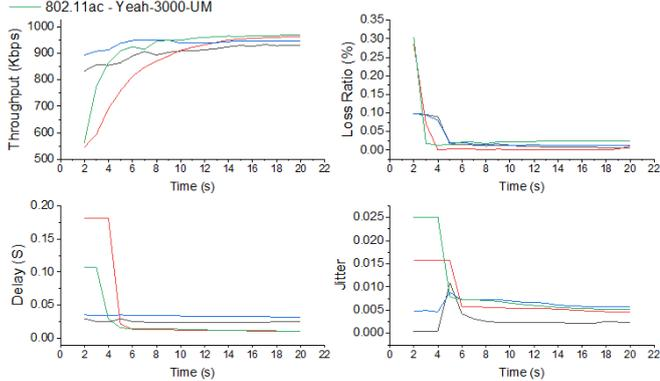
Figure 17: Comparison of loss-delay-based TCP variants in AM mode
