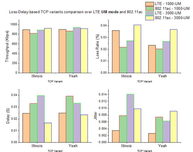
Figure 18: Comparison of loss-delay-based TCP variants in UM mode
