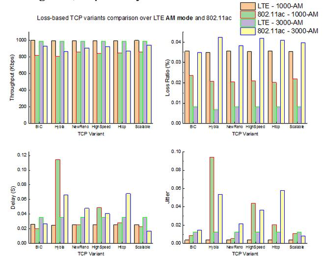
Figure 8: Comparison of loss-based TCP variants in AM mode
