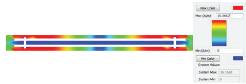
Figure 7: Current flow visualization of Hashtag-shape for DMS at 5.2 GHz
