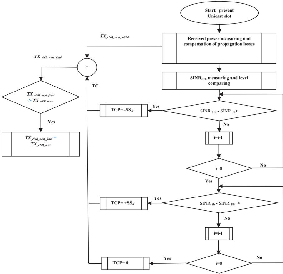
Figure 3: Unicast Slots Power Adjustment Flowchart
