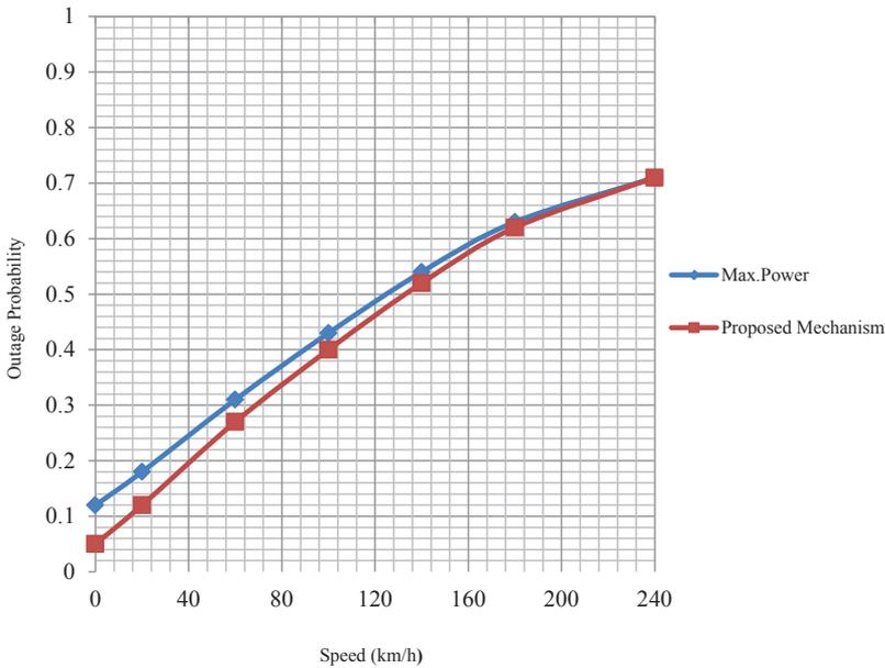
Figure 4: Outage Probability as a function of user speed
