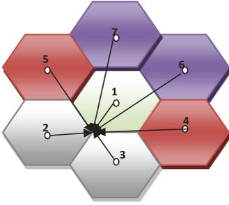
Figure 2: Interference experienced by a cell-edge UE
