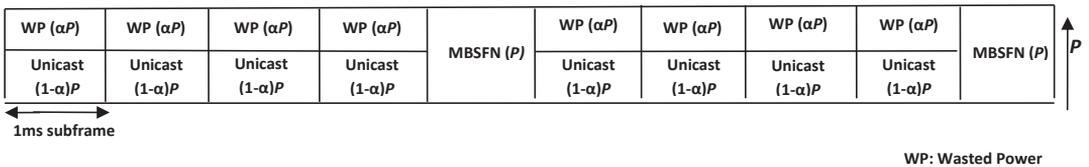
Figure 1: Time Multiplexing between MBSFN and unicast
