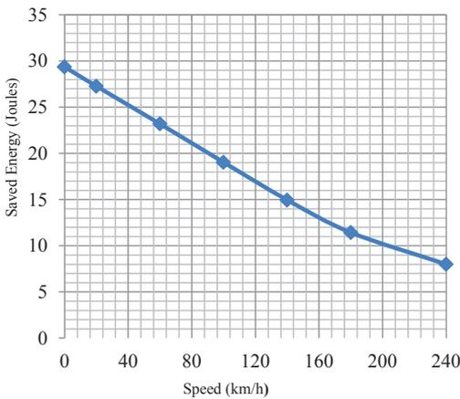
Figure 6: Saved eNB energy as a function of user speed
