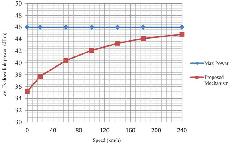
Figure 5: Average Transmitted eNB Power as a function of user speed
