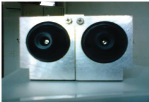
Figure 1: Horizontally aligned of stereo camera.
