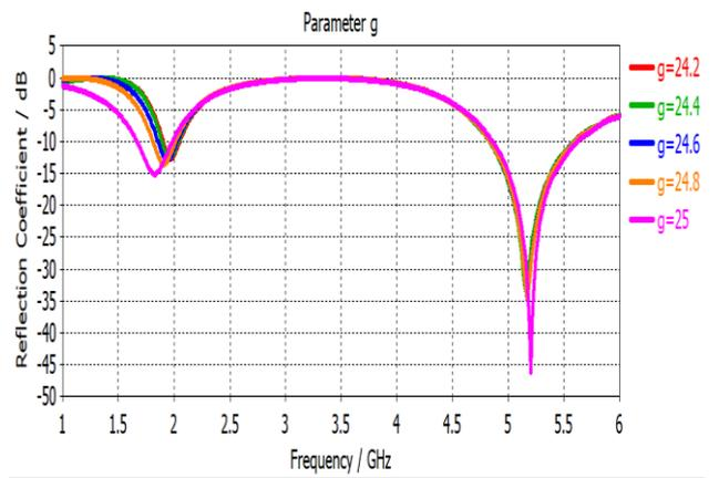
Figure 19: Reflection coefficient analysis of parameter g
