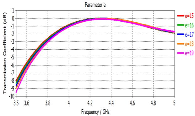
Figure 16: Transmission coefficient analysis of parameter e
