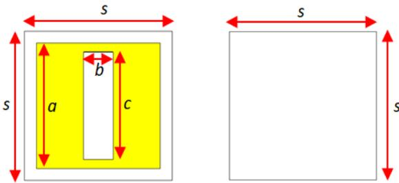
Figure 2: Design B (square patch with rectangular slot)
