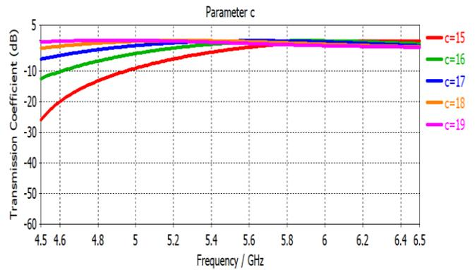
Figure 12: Transmission coefficient analysis of parameter  $c$
