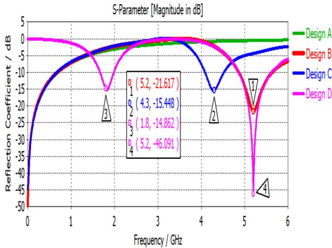
Figure 21: Reflection coefficient (S11) for Design A, Design B, Design C and Design D
