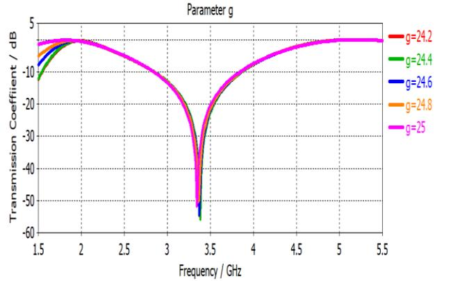
Figure 20: Transmission coefficient analysis of parameter g
