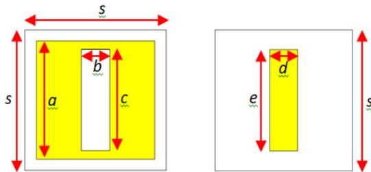
Figure 3: Design C (square patch with a rectangular slot on the glass using complementary techniques)
