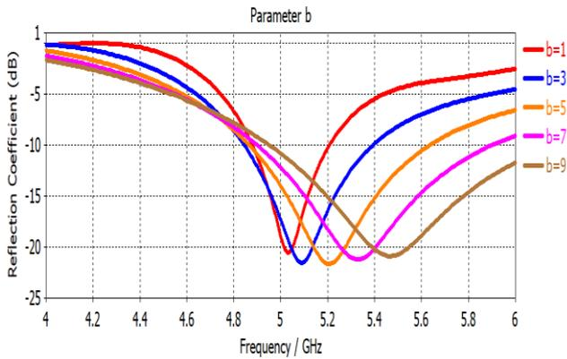
Figure 9: Reflection coefficient analysis of parameter  $b$
