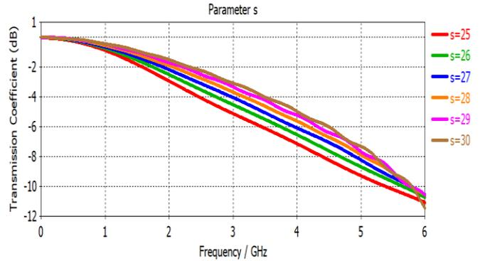
Figure 6: Transmission coefficient analysis of parameter  $s$
