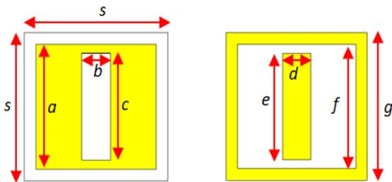
Figure 4: Design D (square patch with rectangular slot and rectangular with a square loop using complementary techniques)
