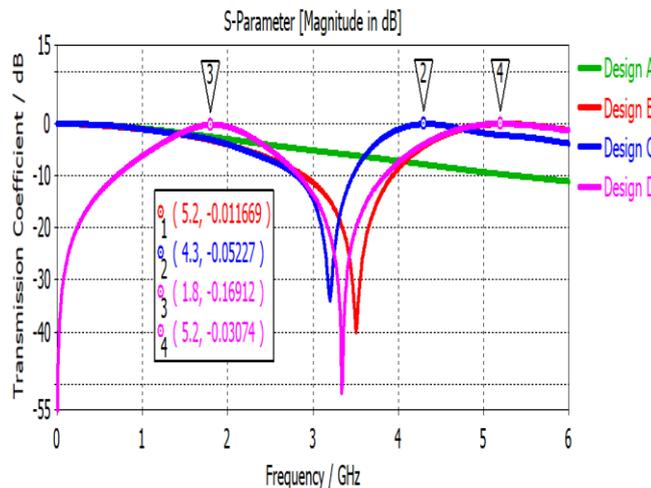
Figure 22: Transmission coefficient (S21) for Design A, Design B, Design C and Design D
