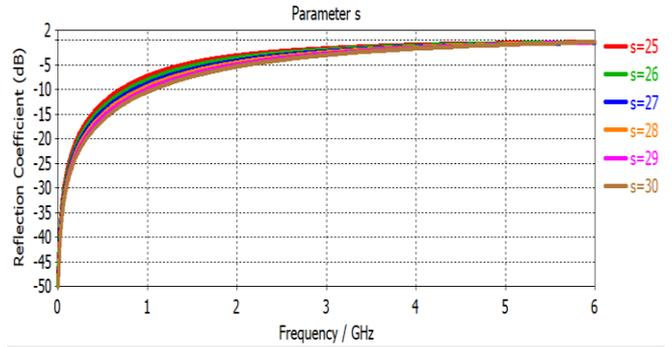
Figure 5: Reflection coefficient analysis of parameter  $s$
