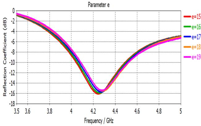
Figure 15: Reflection coefficient analysis of parameter e
