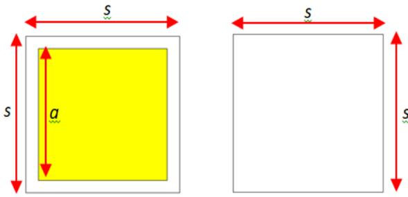
Figure 1: Design A (square patch on the glass)
