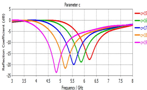
Figure 11: Reflection coefficient analysis of parameter  $c$
