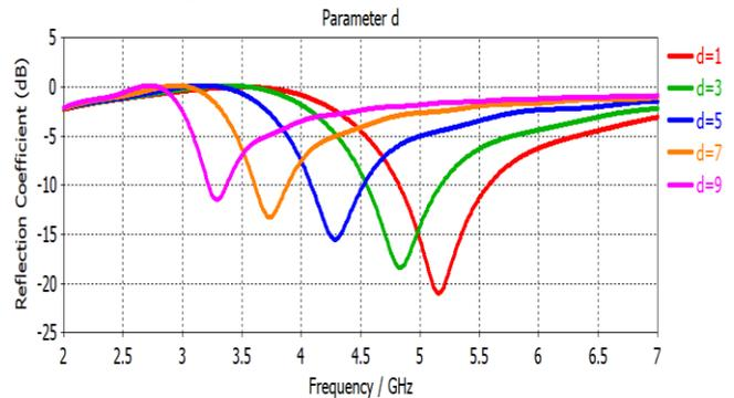
Figure 13: Reflection coefficient analysis of parameter  $d$
