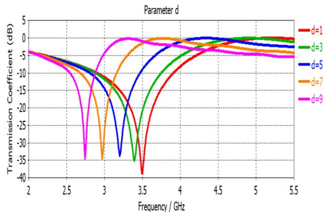
Figure 14: Transmission coefficient analysis of parameter  $d$
