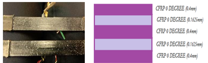
Figure 3: Hybrid Composite CFRP/GFRP
