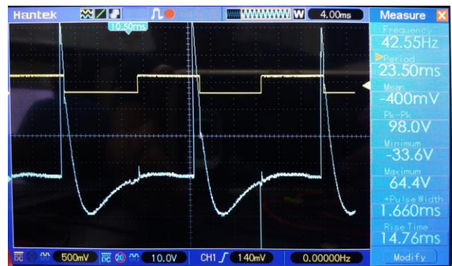
Figure 11: Motor voltage reading in the response of the sensor
